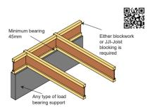
Suitable detailing required if used on an external wall
