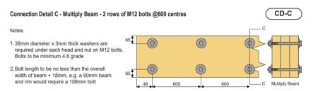
Bolts should be fixed in two rows 65mm in from the top and bottom edge, Bolts should be drilled at Ø12mm and bolts tapped into place. The minimum end distance should be 48mm.
