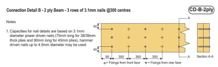
Nails in two ply members should be fixed in two rows 45mm in from the top and bottom edge and one row along the centre line driven from alternate sides. The minimum end distance should be 90mm.
