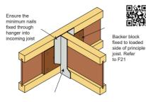
Approved face or top fix hanger secured through specified nail holes (refer to approved connector manufacturer's guidelines
