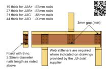
100mm wide plywood, OSB/3 or kiln dried stiffener block fitted to
