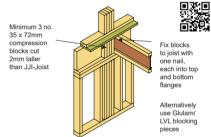
Compression blocks are required where indicated on details provided by JJI-Joist supplier
