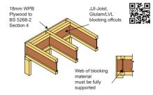
Alternatively use Glulam/LVL blocking in lieu of JJI-Joists JJI-Joist blocking offcuts can be of any joist width
