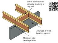
Where split joist(s) of different widths meet on the wall a double row of blocking is required to suit joist widths
