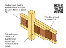
F30-JJI-Joist to steel beam/
