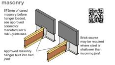
Do not fix joist to steel lintels unless approved by lintel manufacturer Bottom of hanger must rest against bottom flange of steel beam Refer to approved metalwork supplier's literature for further
