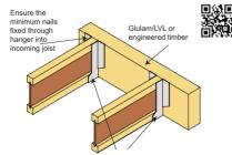
Approved face or top fix hanger secured through specified nail holes (refer to approved connector manufacturer's guidelines
