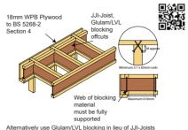
JJI-Joist blocking offcuts can be of any joist width
