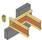
JJI-Joist nogging/ dwang min 45mm wide flange (or timber min 38 x 45mm) securely fixed with 3.35 x 65mm skew nailing or
