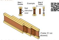
Provide filler blocks at all ends and bearings of joist and at points of incoming loads (see F15). Alternatively provide continuous filler block when repeated loads are applied (see F40)
