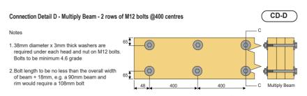
Bolts should be fixed in two rows 65mm in from the top and bottom edge, Bolts should be drilled at Ø12mm and bolts tapped into place. The minimum end distance should be 48mm.
