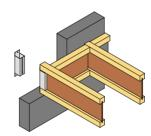
JJI-Joist nogging/ dwang min 45mm wide flange
