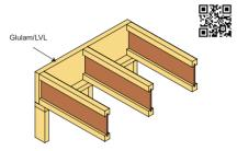
Additional blocking may be required to Engineer's specification, to improve sound, structural performance and fixing
