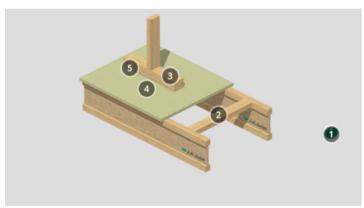
F4 | Non-load bearing wall parallel to Joists
