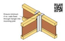
Approved backer free hanger secured through specified nail holes Refer to approved connector manufacturer's guidelines
