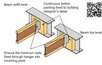
Approved face fixed hangers fixed through all nail holes Refer to approved metal work supplier's literature for further
