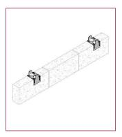
Gable restraint brackets placed on wall at 1200mm\* maximum centres (no fixings required).
