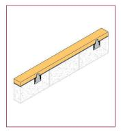
38-75mm wallplate bedded on mortar and fixed to gable restraint brackets with 3.5x40mm wood screws (2 no. per bracket).
