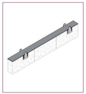
10mm maximum mortar bed on wall prior to wallplate being fixed.
