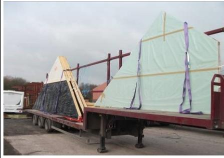
3. The clad panels are individually attached to the centre bar of the trailer with blue rope to the sacrificial white straps. **White straps are not the lifting point.**
