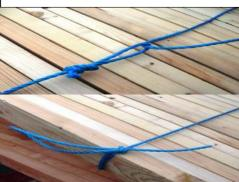
6.The loader must secure each pack to the centre bars with blue rope at minimum two points above the centre of gravity of the truss pack.
