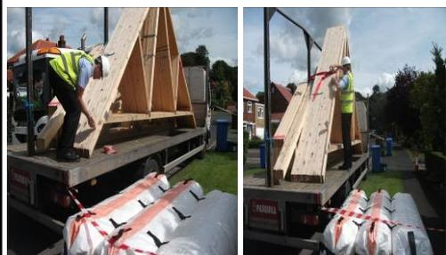
9. The customer shall place his team to receive the truss. The customer shall remove the truss from the vehicle. The driver will repeat this method by releasing one truss only.
