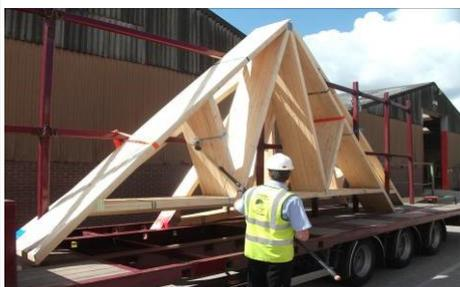
8. The driver will apply a wedge between the 1st and 2nd truss. The driver will then re-fit one of the small straps through the gap to secure the pack but leaving one to be taken by the customer.
