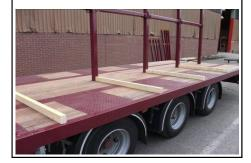
4. On instruction from the site responsible person the driver will release the transport straps on the side being unloaded ensuring no one is within the danger area as shown in the pictures.
